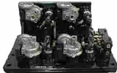
Hydraulic operated clamping fixture with two "Op. A" & two "Op B" workpieces.
